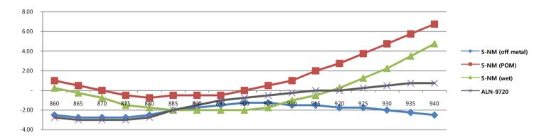
•SMALLEST NM reads 3.5 meters in US band, 20% longer than ALN-9720. Covering both EU and US band, It is best performing off metal tag among similar sized UHF tags. And no similar size tag shows gentle and stable curve slope across EU and US band as SMALLEST NM shows.
